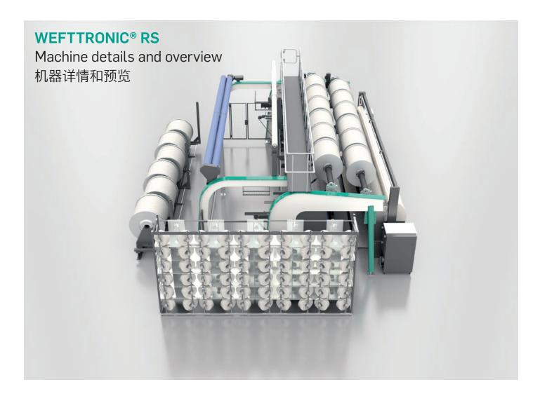
The WEFTTRONIC® RS is a Raschel machine with parallel weft insertion which is operated with up to three guide bars depending on the application.
