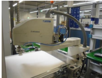
Check of mirror position by a Robot-Vision-System
