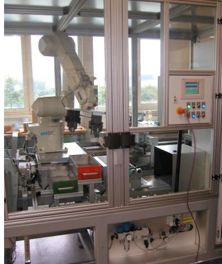
Optical true running control of sintered hard metal sticks Radial run-out less than 0,1 mm
